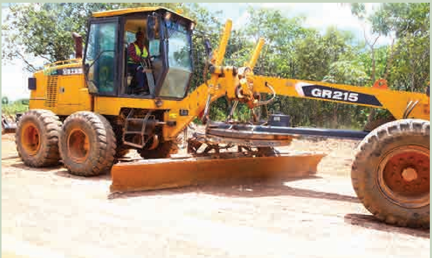
Grader Operator working on the Lubambe emergency access road.
