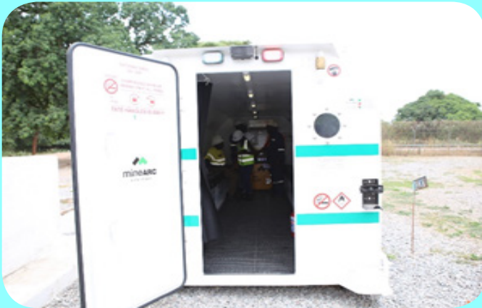
Inside and outside of one of the five newly procured refuge chambers
